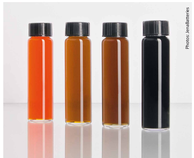
(Left to right): uncharged catholyte, charged catholyte, uncharged anolyte, charged anolyte. The organic electrolytes change color depending on their charge state.
